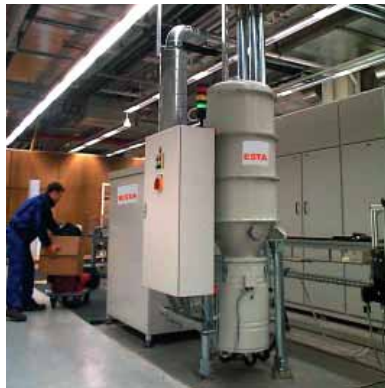
Cyclonic filter FZ-1003 with 100 Litre collection container
