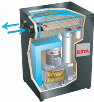
Schematic illustration of a side channel blower with direct drive
