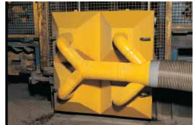
Large surface extraction hood in the concrete industry
