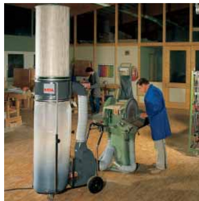
Mobile extraction unit with cartridge filter
