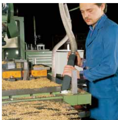
Clean up of brass chips and coolants at a CNC milling station
