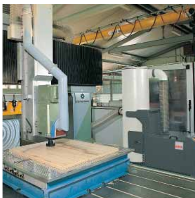
DUSTOVAC extracting at a CNC controlled machine
