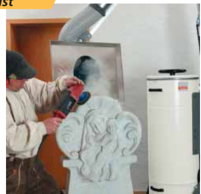
DUSTOMAT-16 M – direct extraction of fine stone dust
