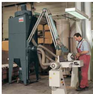
Wet separator NA-K extracting aluminium dust
