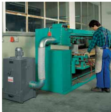
OM-12 connected to a surface finishing machine
