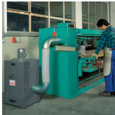
Mini dust collector OM connected to a surface finishing machine
