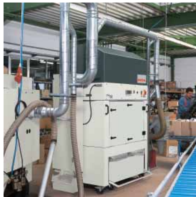
Compact dust extractor model COMPEX in the shoe industry
