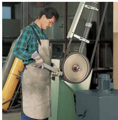
OMF connected to a belt sanding machine
