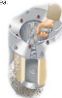
Cleaning with compressed air
