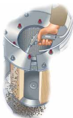
Cleaning with compressed air
